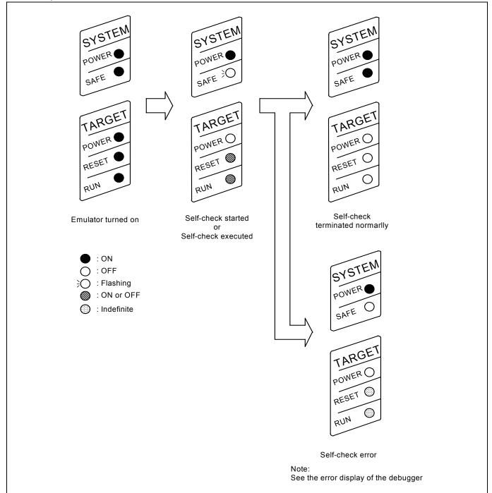
Figure 2.6 LED displays during the self-check
